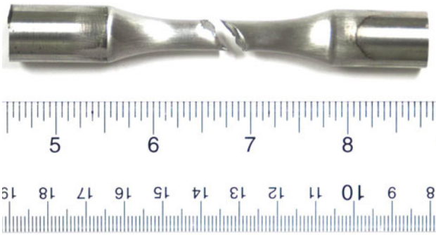
Fig. 15 Optical image of 45° fatigue crack orientation in profile view of sample Q17 tested at a \epsilon_a of 1% with N_f of 1,029
