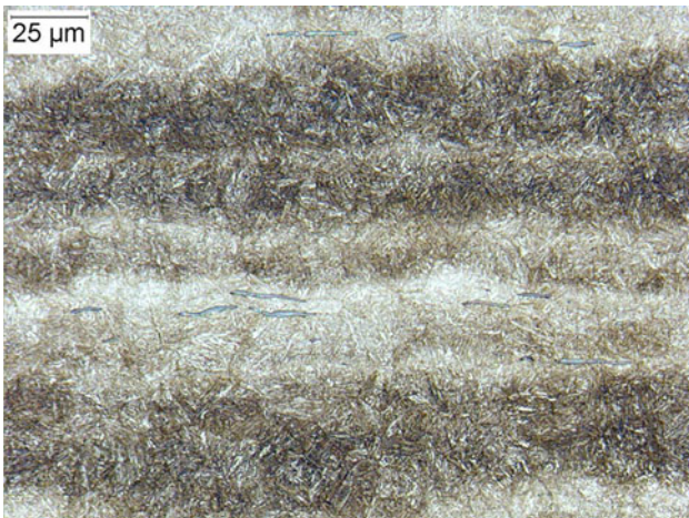
Fig. 5 Optical micrograph of longitudinal section of Q&T sample
